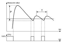
Fig.12. Selection of settings by the oscillation method. Calculate controller settings acc. to given formulas: Pb = P ti = T
