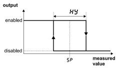
Fig.10. Operation way of the heating type output
