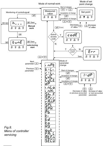
The access to parameters can be protected by a code. If the safety code is set (parameter **SECU** is higher than zero), one must give it. If the value will not be given or will be erroneous, the inscription *Err* appears on displays, and the user will be only able to monitor parameter values.
