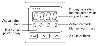
Fig.6. View of the controller frontal plate.
